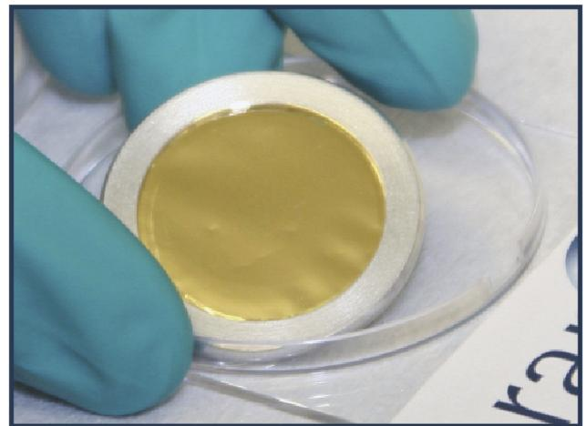
Fig. 1: filtr.AID Membrane in Petri Slide. Gold-plated, aluminum-mounted polycarbonate membrane.
