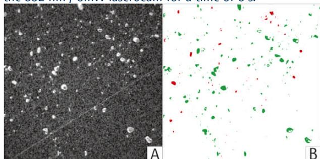
Figure 1: DF Microscopic image (500 µm x 500 µm (A)). B: Image analysis result of the same image. (Liquid Particle Explorer) green=lactose ; red=tolmetin (analysis time = 100 seconds)
