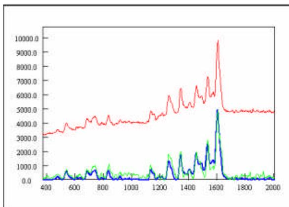
Figure 2: 5s exposure original spectra of one tolmetin particle (red), proceeding spectra (blue) match with Rank: 957 = tolmetin library spectrum (green)
