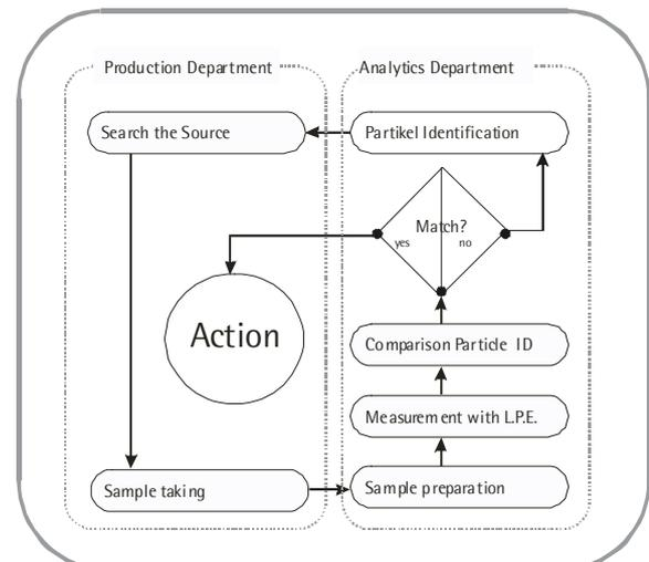
After the identification of the material with the automated Raman spectroscopy it is very important for final verification of the result to track down the assumed source of the contamination in the production process and to obtain its spectrum, too. After successful allocation the new spectra from the material sample will be added to the database with a mouse click. These additional data will be the best possible basis of the future supervision.
