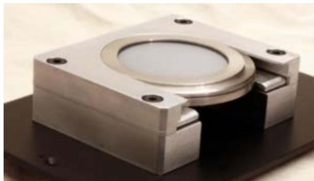
Fig.2: Wet cell in a sample holder, layer thickness was set to 400 µm resulting in a sample volume of 700 µL
